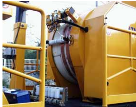
Cable clamping device, fit for 1, 2, 3 or 4 cables
