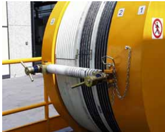
Roller for pressing 1, 2, 3 or 4 cables
