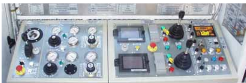
CONTROL PANEL OF MACHINE WITH 2 CIRCUITS AND 2 REEL-STANDS
