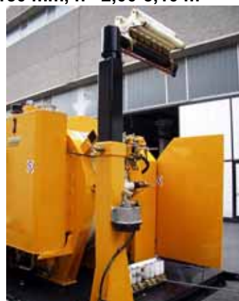
Telescopic mast, sq. 150 mm, h= 2,00-3,10 m
