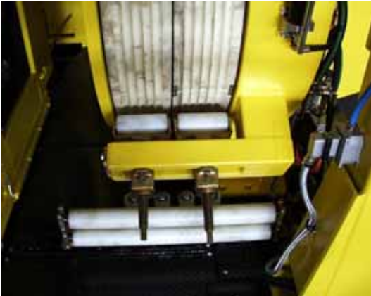
Roller for pressing 2 cables
