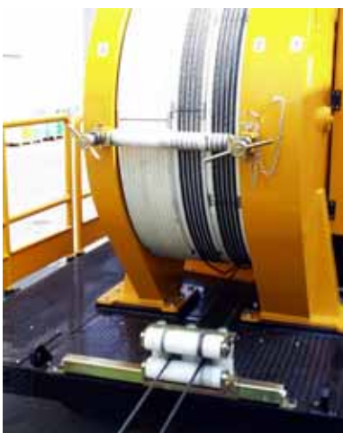
Cable-driver for 2 cables
