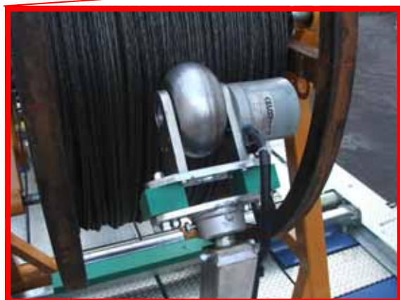
DEVICE TO CHECK THE QUANTITY OF CABLE WINDED ON THE REEL
