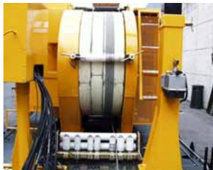
Cable-driver for 4 cables
