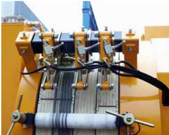
Cable clamping device, fit for 1, 2, 3 or 4 cables
