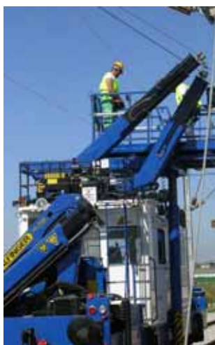
Telescopic fingers, independent, equipped with rollers and radio controlled
