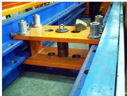
Second trolley with pins (Bench capacity 100 Ton)
