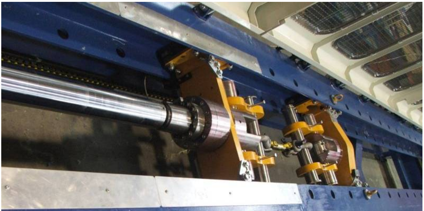
Traction and reaction trolleys (Bench capacity 60 Ton)
