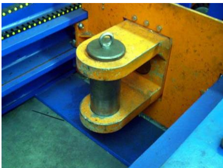
Traction trolley with hook (Bench capacity 150 Ton)
