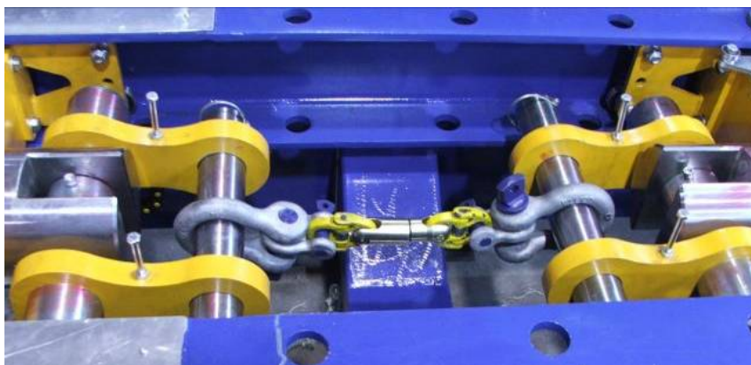
Special forks, adjustable in width
